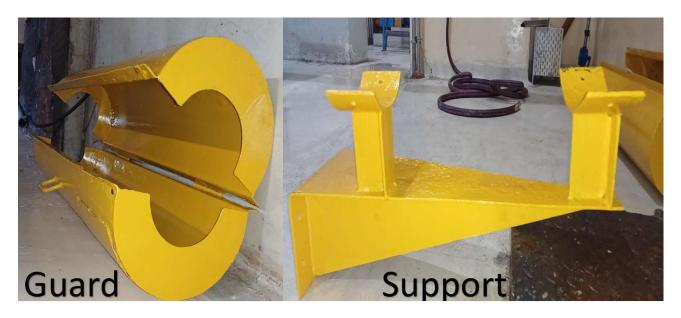
2. Shaft guard and support frame for Short former; MOC: SS 316 L
