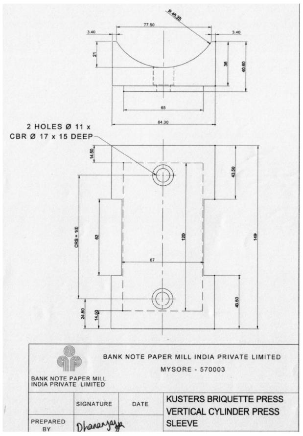
14. Supply of Wear guide block for briquette press vertical cylinder, MOC: Brass
